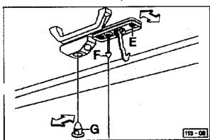
After the position of the pop up roof was changed, it must be examined whether the sole plate can still be hung up into the owner. The situation of the owner can be adapted after loosening of the screws. *Torque data:* **8.3** Nm
